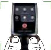
Professional zoom wheel with excellent build quality gives finer control over progressive zoom speeds. Zoom wheel direction can be inverted (left – right or right – left).
