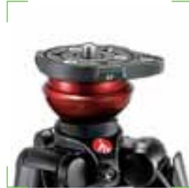
Tripod to head connection via a disc with 3/8" male thread, built-in spirit level and three grub screws for secure locking mountings.
