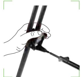
To open the spreader, press the ratchet pin and pull the leg outwards to the desired click stop.
