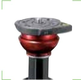
Centre column with built-in 50mm half ball locked using the rotating grip located at the bottom of the centre column. Tilt range: +15°/-15°.
