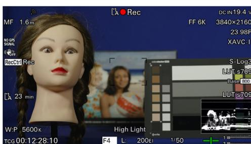
Exposure is adjusted 2 stops brighter to bring brightness to MLUT image to the same base setting. The recording becomes brighter as a result
